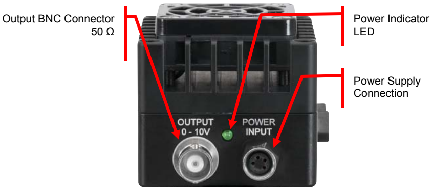
Figure 1 Electrical Connections
